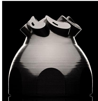
A marine burner atomizer (close-up, left, after installation, below) made using 3D printing techniques. It cannot be manufactured using traditional machining methods.
